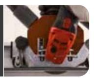
For L-shaped cuts or cuts within the slab, holes must be drilled at the vertexes so that the slab does not break during or after laying.
