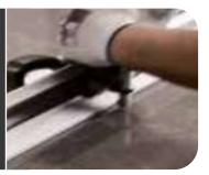
To cut the slab without breaking the material, the appropriate shears should be used.
